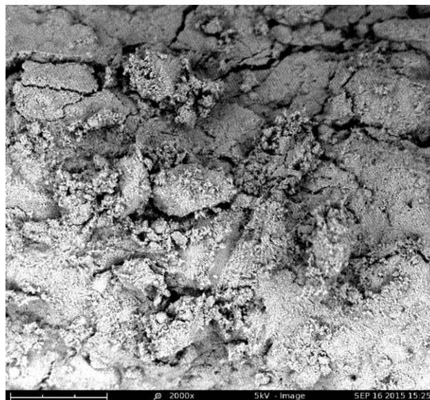
Figure 3: SEM micrograph of the 150 oC annealed CuO sample
