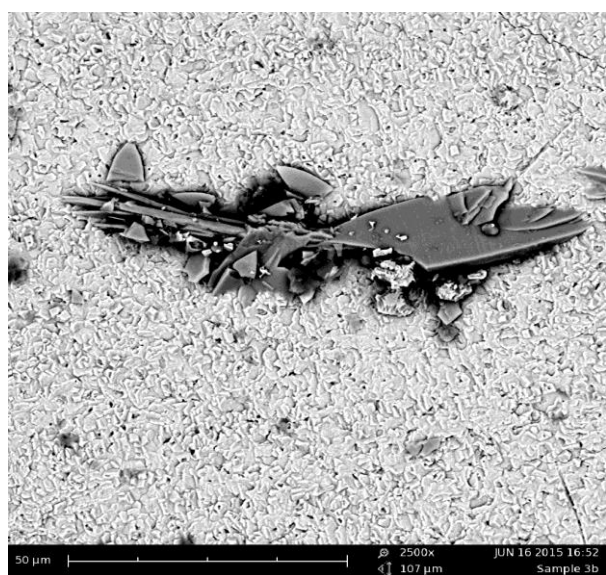
Plate 2: SEM micrographs of the un-annealed sample prepared by immersion with a solution of 0.001M \text{CuSO}_4 for a period of 36 days.
