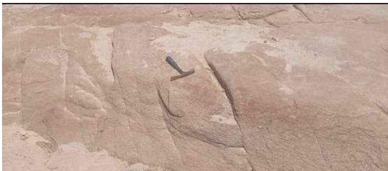
Figure 21: Medium-coarse-grained granite exhibiting some systematic joints in Mahangi; Latitude 11° 14' 38"N and Longitude 08° 15' 21"E.
