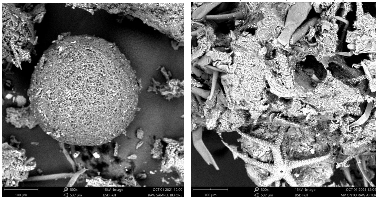
(a) (b) Fig 2: SEM micrograph (a) before adsorption of MG (b) after Adsorption of MG
