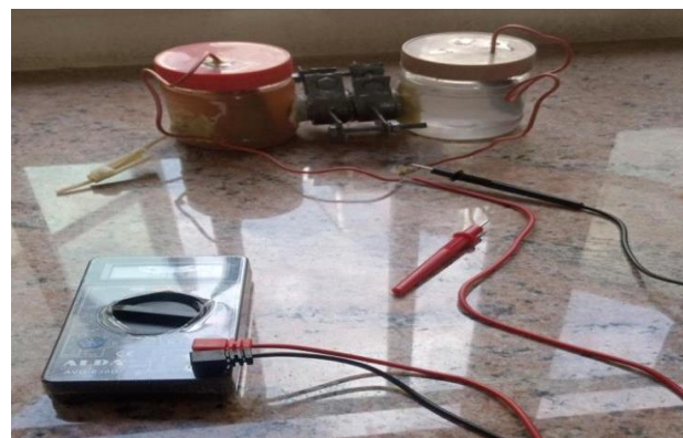
Figure 1: Two Chamber MFC utilized for this work
