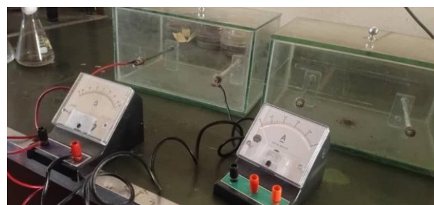
Plate 2: Single Chamber Microfuel Cell connected to Ammeter and Galvanometer
