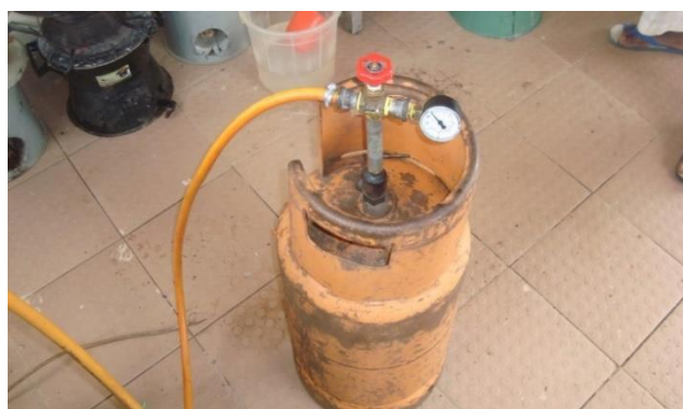
Plate 8: Compressed Natural Gas (CNG) Cylinder with Pressure Gauge
