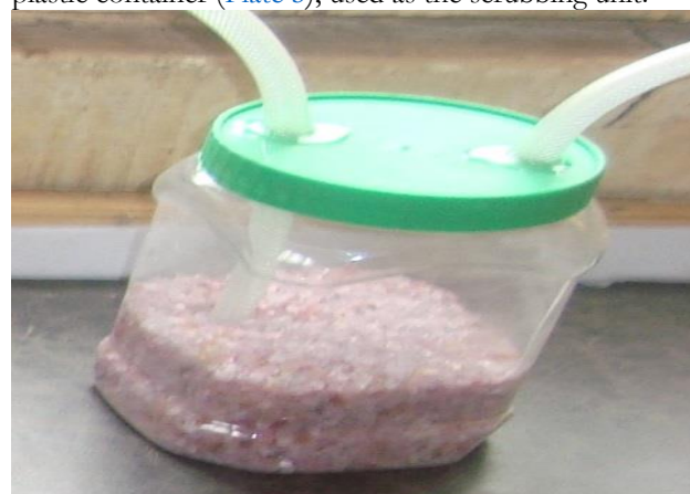
Plate 5: Silical gel Crystals for scrubbing water vapour
