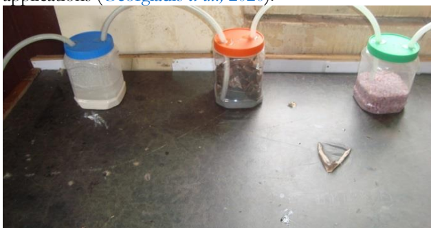
Plate 2: Biogas scrubbing units set-up
