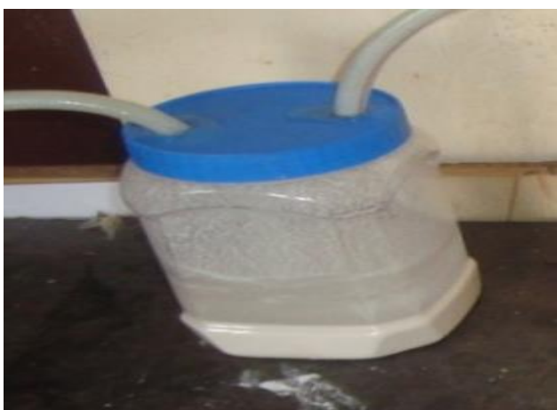
Plate 3: Calcium oxide container for scrubbing CO 2
