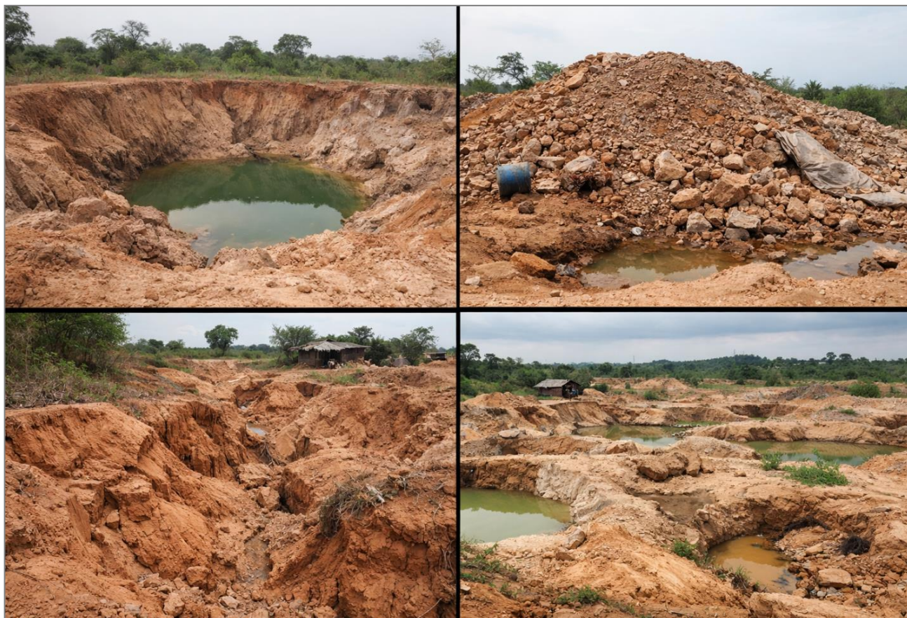
Plate 1: Representative field photographs showing abandoned pits, spoil heaps, and erosion features at artisanal mining sites in Oke-Ogun.
