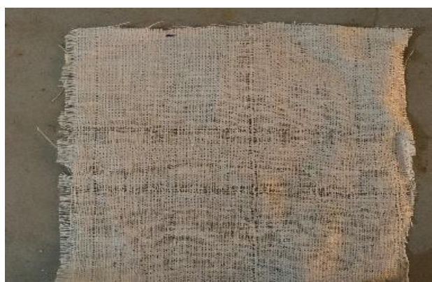
Figure 2: Woven kenaf preform
