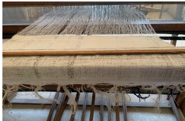
Figure 1: Weaving kenaf preform using a floor loom
