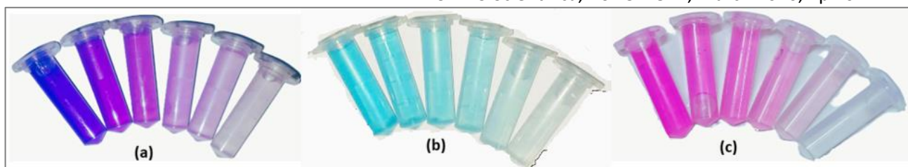
Figure 5: Photographic images showing the visible-light-driven degradation of (a) crystal violet (CV), (b) methylene blue (MB), and (c) rhodamine B (RhB) using the BaTiO 3 /Co-ZnO (S3) photocatalyst at different irradiation times.
