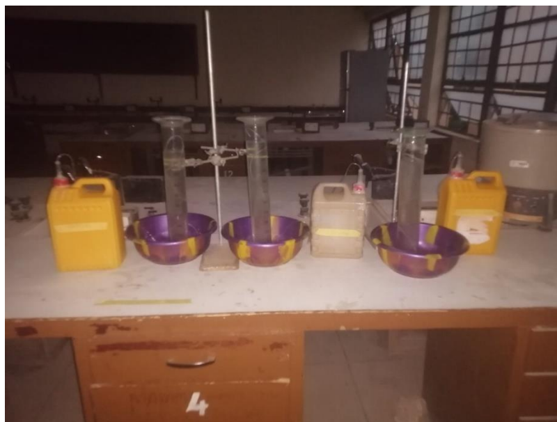
Plate I: Experimental Set-up for the Anaerobic Digestion of Municipal Organic Wastes
