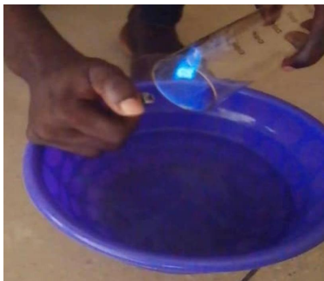
Plate III: Flammability (Quality) Test for Methane Content of the Set-up with Non-activated Carbon Supplementation
